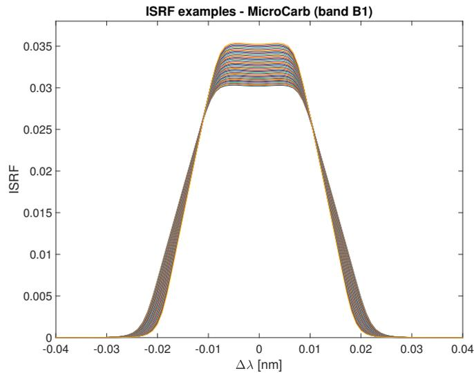
**Figure 1.** Illustration of a superposition of 1024 ISRFs with centered wavelengths  $\lambda_l = 758.3, \dots, 768.3$ nm around their central wavelengths. The ISRFs have been simulated for the band B1 of the MicroCarb instrument using uniform scenes.
