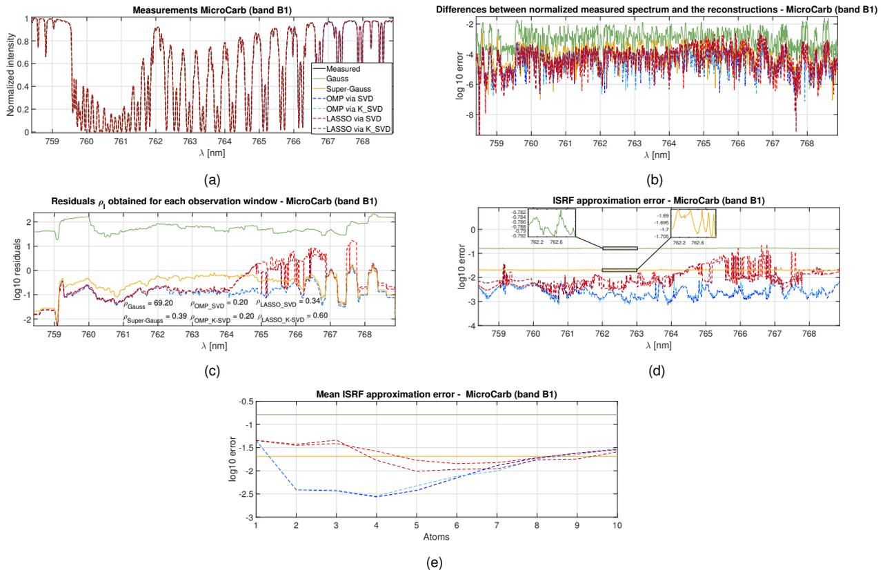
**Figure 5.** Illustrations of a) the measured spectrum reconstruction, b) the difference between the measured spectrum and the reconstructed ones, c) the residuals  $\rho_i$  for each wavelengths, d) the ISRF approximation error versus the wavelength and e) the mean ISRF approximation error versus the number of selected atoms for different methods (Gauss, Super-Gauss, OMP, LASSO, SVD and K-SVD) and for the band B1 of the MicroCarb instrument.
