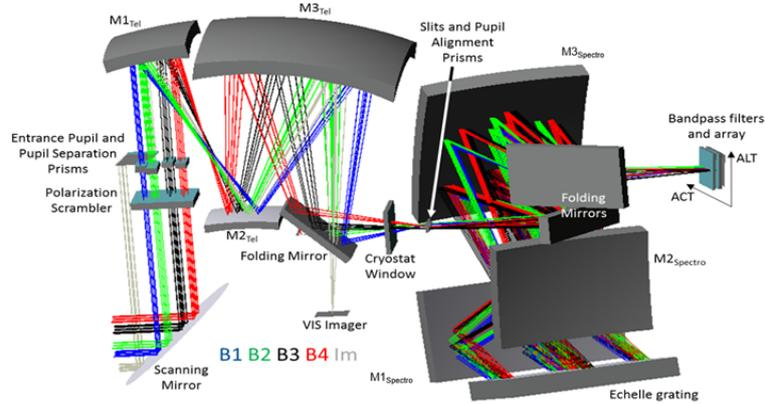
**Figure 3.** Principle design of the MicroCarb instrument reproduced from (Castelneau et al., 2019).
