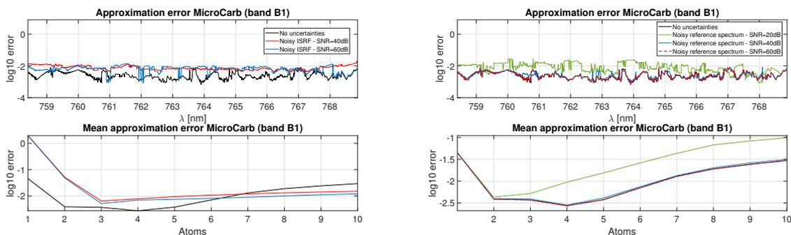
**Figure 16.** Results obtained using SVD and OMP for the different scenarios of noisy ISRFs in the construction of the dictionary (left) and noisy reference spectra (right) for the band B1 of MicroCarb.
