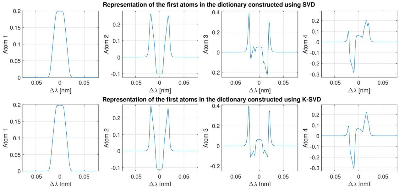
**Figure 2.** Representation of the four first atoms of the dictionary of ISRFs  $\Phi$  constructed using an SVD on the matrix of representative ISRFs (top) or using the K-SVD algorithm using the same matrix of representative ISRFs (bottom) for the MicroCarb spectrometer (band B1).
