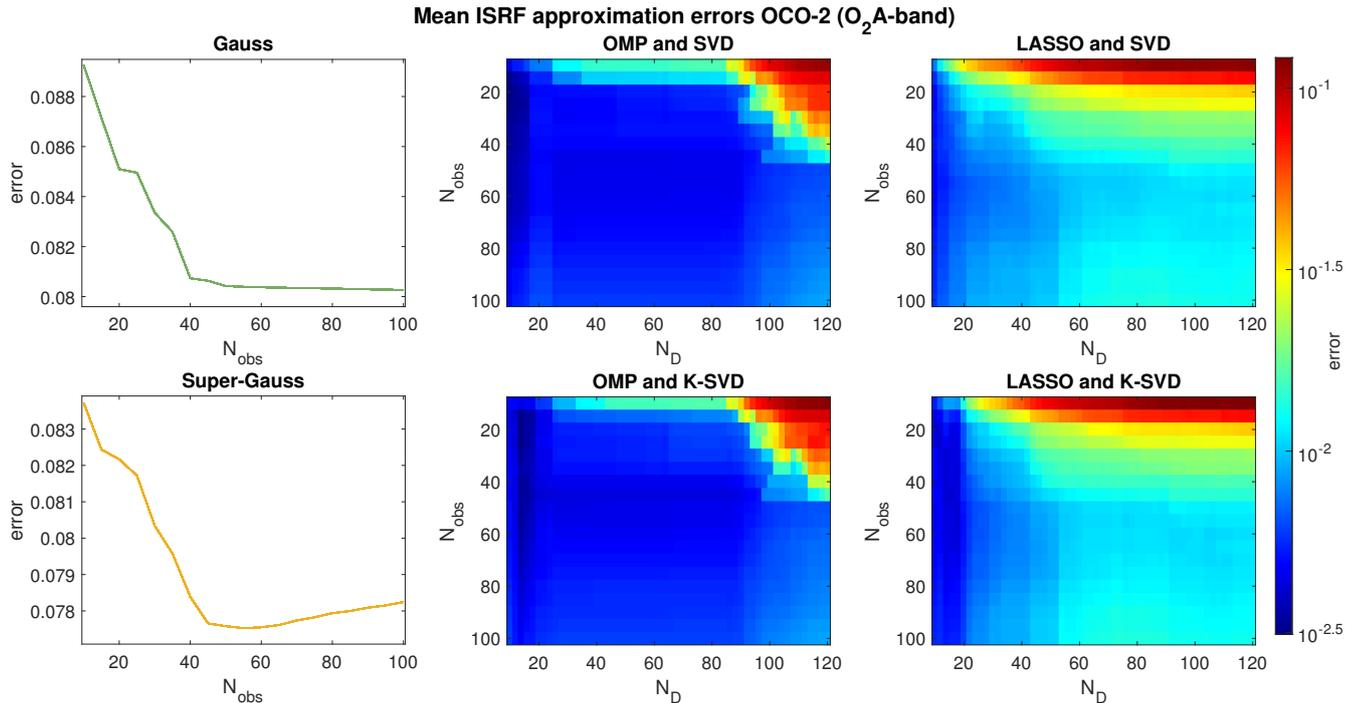
**Figure 9.** Mean approximation errors for OCO-2 and the different estimation methods (Gauss, Super-Gauss, OMP and LASSO with SVD or K-SVD) versus the number of observations  $N_{\text{obs}}$  and the dictionary size  $N_D$  for  $K = 5$ .
