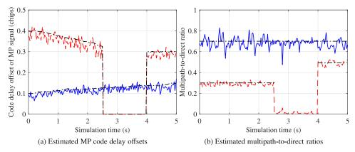
Fig. 8. Estimation results for two MP signal parameters in dynamic scenarios. MP #1: blue solid line; MP #2: red dashed line; True value: black dash-dotted line. (For interpretation of the references to colour in this figure legend, the reader is referred to the web version of this article.)
