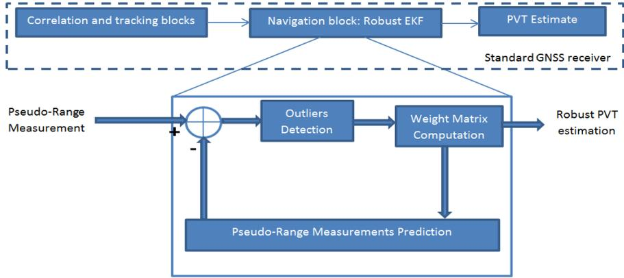
Fig. 1. High-level block diagram of the Adaptive Robust Extended Kalman Filter estimator
