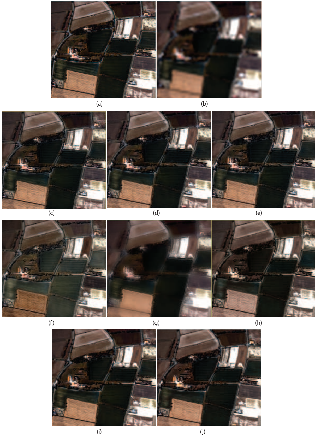
Fig. 1: Details of original and fused Camargue dataset HS image. (a) reference image, (b) HS image interpolated, (c) SFIM, (d) MTF GLP HPM, (e) GSA, (f) PCA, (g) GFPCA, (h) CNMF, (i) Bayesian Sparse, (j) HySure
