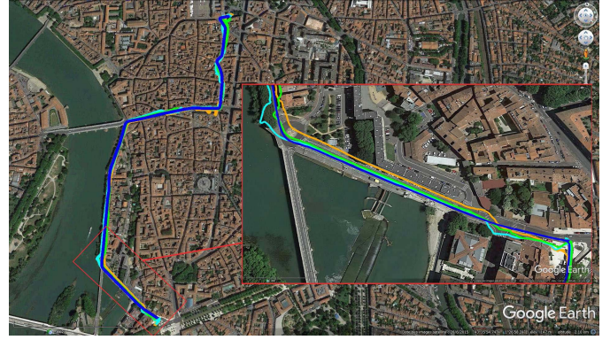
Fig. 20. Trajectory of the urban scenario plotted using Google Earth ® . The reference is in blue, the Ublox and REKF solutions are in green and orange, whereas the proposed method is in cyan.
