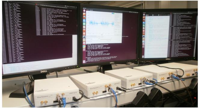
**Figure 1:** All our experiments are carried out on a five-node USRP N210 testbed.
