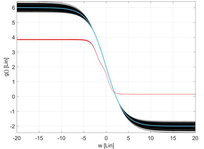
**Fig. 6.** Estimated nonlinearity  $\hat{g}(\cdot)$  obtained with the MLEs (13a-13b, in black) and Pawlak's estimators (2a, in red) of  $(\lambda, \alpha, \beta)$ , compared to the ground truth  $g(\cdot)$  (in blue) at  $SNR = 52dB$ .
