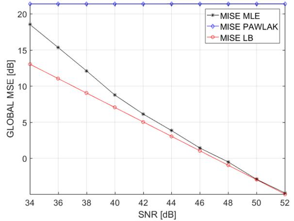
**Fig. 5.**  $MISE(\hat{g}(\cdot))$  (10) of the MLE (13a-13b) and of Pawlak's estimator (2a) versus SNR, compared with the lower bound (11).
