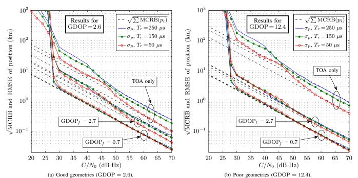
Fig. 4. Estimation of beacon position for (a) good geometries and (b) poor geometries considering different values of the rise times  $T_r$  and  $\mathrm{GDOP}_f$ .
